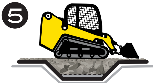
5 FINE GRADE ENTIRE ROAD
